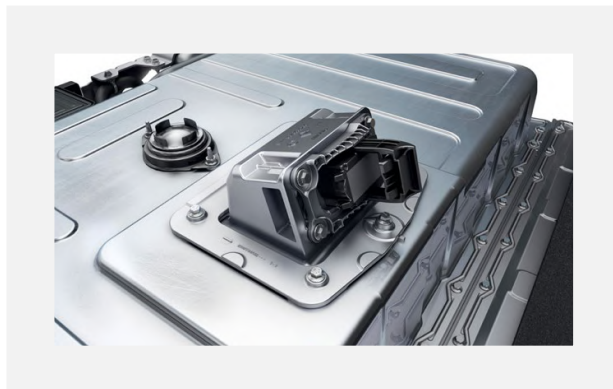
Figure 1. Traction battery Electric Renault Megane E- Tech with the Fireman Access system and the service plug
